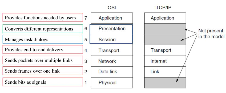
Figure 1-21. The TCP/IP reference model.
