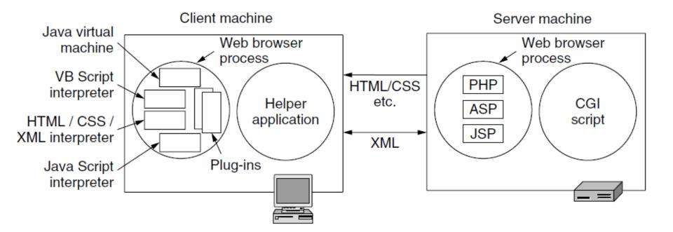
Figure 7-35. Various technologies used to generate dynamic pages.
